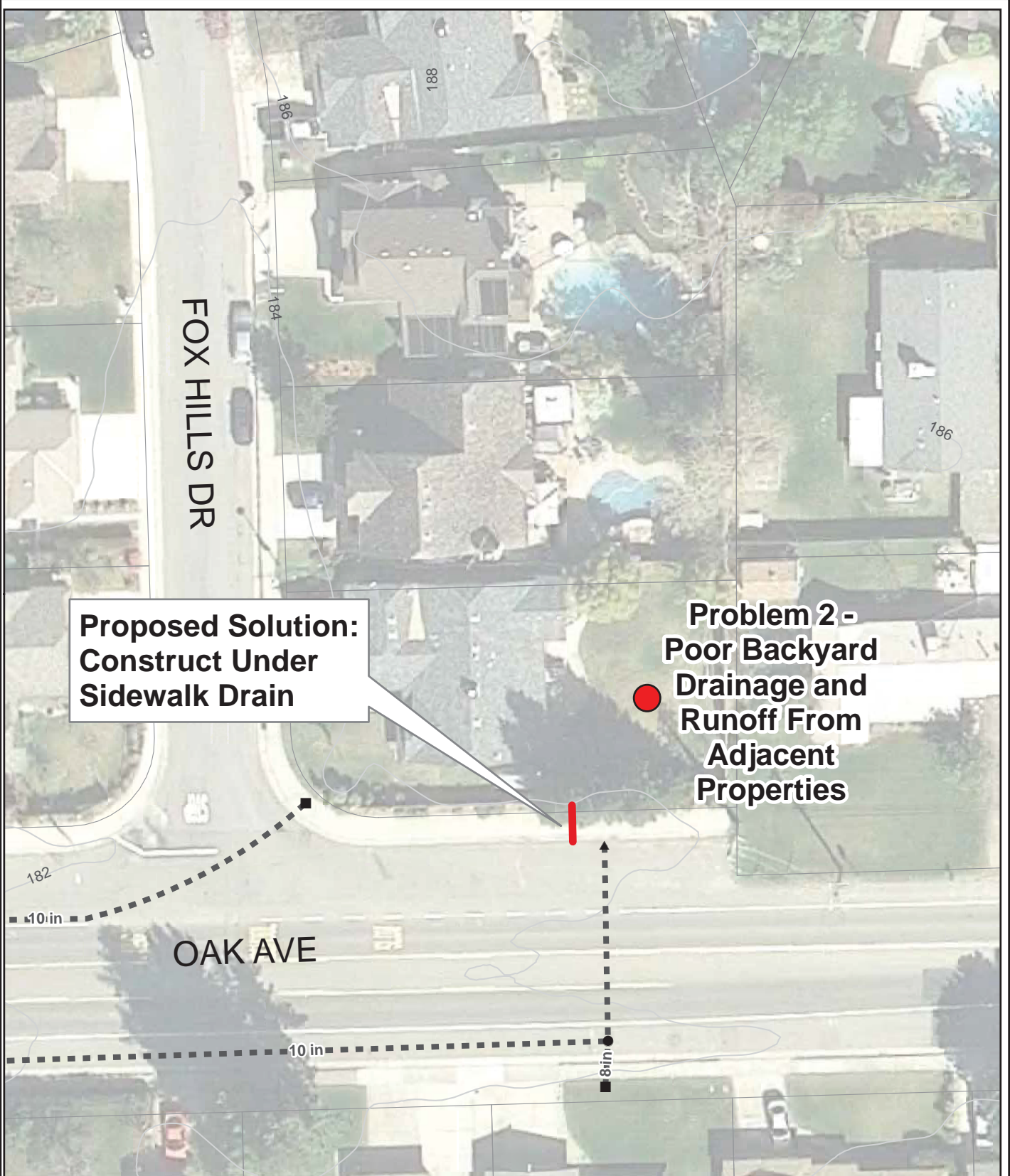
Figure 7-3 City of Citrus Heights Neighborhoods 8, 9, and 10 Drainage Master Plan Study Problem Location 2 and Proposed Solution
