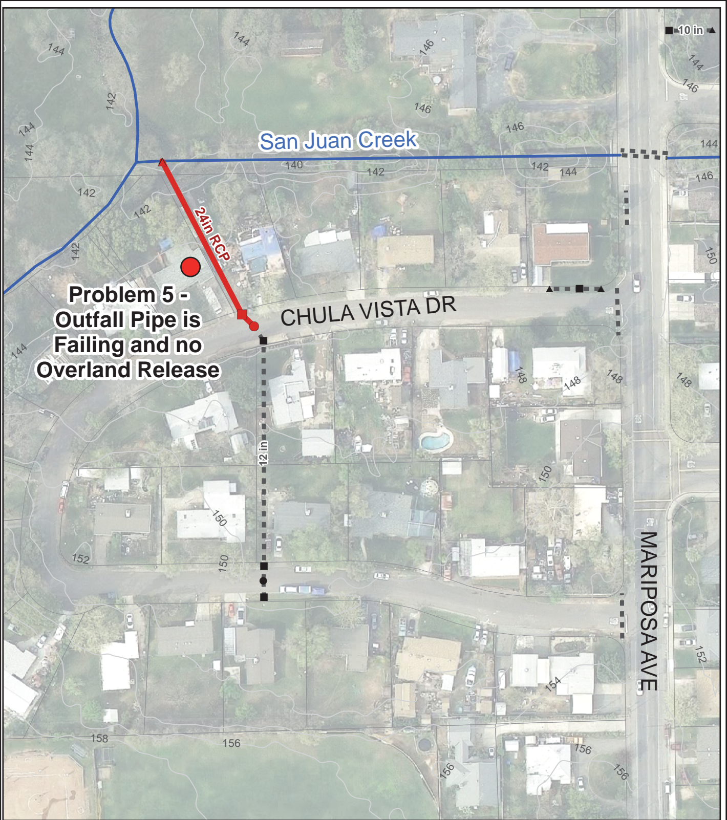
Figure 7-6 City of Citrus Heights Neighborhoods 8, 9, and 10 Drainage Master Plan Study Problem Location 5 and Proposed Solution
